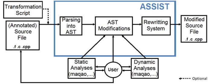
Fig. 1. Overview of the ASSIST process. The user decides what static and dynamic analyses have to be performed.
