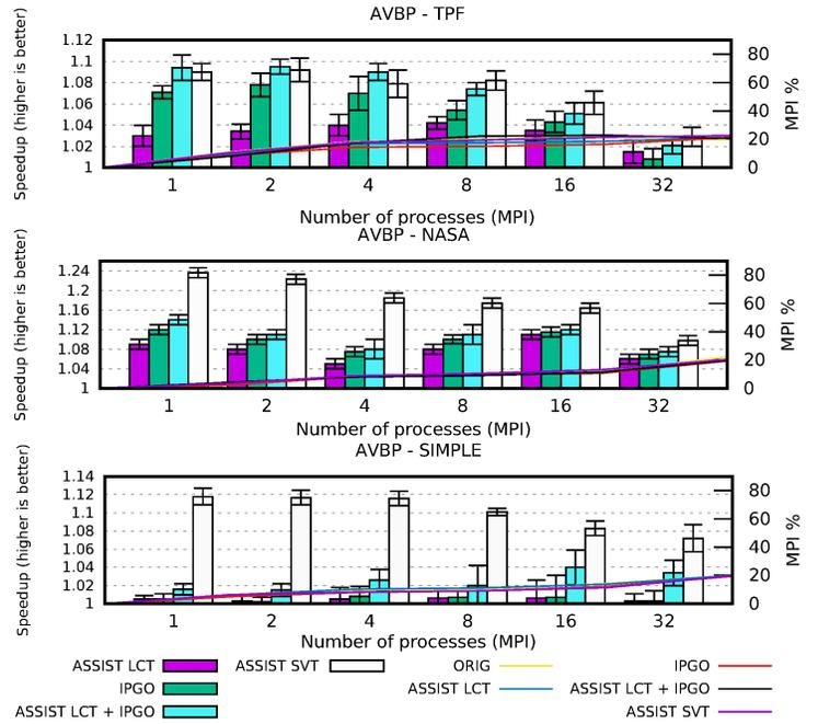
Fig. 6. **Histograms**: Speedups of ASSIST SVT & LCT, IPGO and ASSIST LCT + IPGO compared with the original version (higher is better) on three AVBP datasets. **Plots**: Percentage of execution time spent in MPI.
