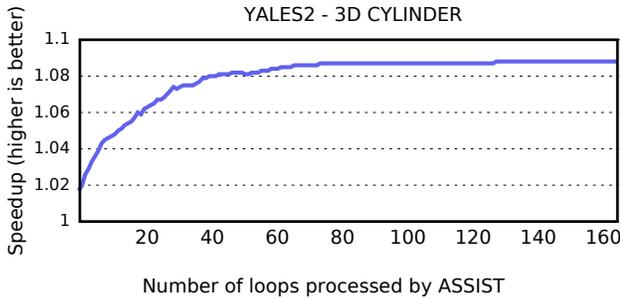
Fig. 4. Cumulated speedup versus number of loops processed by ASSIST, sorted by coverage, on Yales2 using the 3D Cylinder test case.
