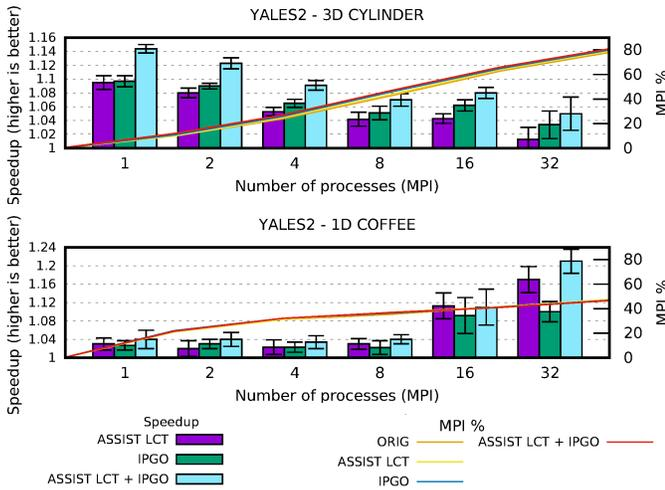
Fig. 3. **Histograms:** impact (speedup) of ASSIST LCT, IPGO and combination of both compared with original version for the same number of threads of two datasets Yales2 (Higher is better). **Error bars** represent original version / minimum speedup and original version / maximum speedup. **Plots:** Percentage of execution time spent in MPI.
