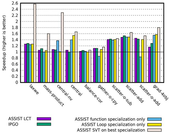
Fig. 5. Speedups by function before and after applying transformations with ASSIST (SVT, function/loop specialization, LCT) and IGO compared with the original version (higher is better) on AVBP using the SIMPLE test case (sequential version).
