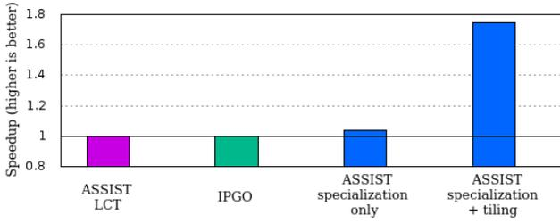
Fig. 7. ABINIT - Ti-256 - Speedups of IPGO, ASSIST LCT, specialized with ASSIST, specialized and tiled with ASSIST compared to the original version
